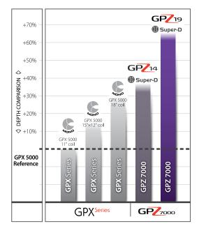
In iron mineralised ground, a GPZ 7000 detector with a GPZ 19 coil will achieve much better results than a GPX Series detector with any size Commander coil. In very salty ground the GPZ 14 coil may give better results than the GPZ 19 coil. I Refer to www.minelab.com or product carton for further details
